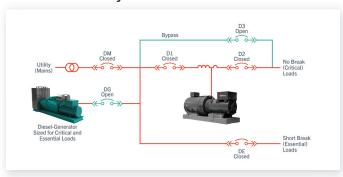
When the Utility supply returns, the VFD, via the drive motor of the Rotabloc, ensures that the Flywheel is recharged. Once the Rotabloc is fully charged, the Utility Breaker N1 closes and the load on the EG is reduced gradually before the Generator Breaker G1 is opened to disconnect the Genset. During this transfer all loads are maintained without a break.
