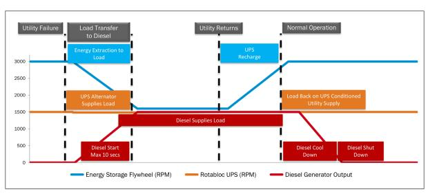
Note how, after a programmed 'hold' of up to one second, the Critical Load is transferred quickly from the failed Utility to the back-up Diesel Genset.
