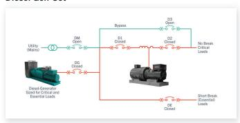
After a short period of serving only the 'No-Break' loads, Breaker D1 closes and reconnects the 'Short-Break' loads. The VFD then maintains the Flywheel at a fixed speed, or recharges it, dependent on EG rating. During this period all loads remain connected.
