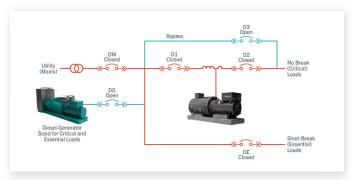
In Normal Operation, the Rotabloc filters the supply to the 'No-Break' loads and regulates the power factor at the Utility service input. This means that all equipment is protected against variations in power quality and assets that require continuous power are always secure from interruption.
