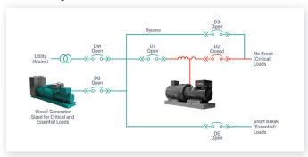
When the Utility fails, N1 and D1 open and the Engine Generator (EG) receives a 'start' signal. During the EG start period the Rotabloc discharges into the 'No-Break' load to maintain power, whilst the 'Short-Break' loads are disconnected. When the Generator comes fully up to speed, the diesel syncs with the UPS and then G1 closes. All 'No-Break' loads are maintained during this period.
